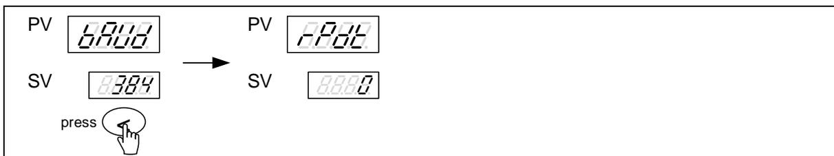
14. Press SHIFT key then lower display will start flash, press UP key or DOWN key to select communication response delay time(ms) then pressing SET key to save the current setting.
