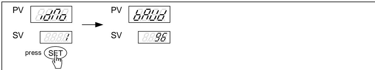
12. Press SHIFT key then lower display will start flash, press UP key or DOWN key to select baud rate then pressing SET key to save the current setting.
