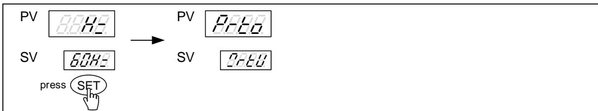
6. Press SHIFT key then lower display will start flash, press UP key or DOWN key to select communication protocol then pressing SET key to save the current setting.
