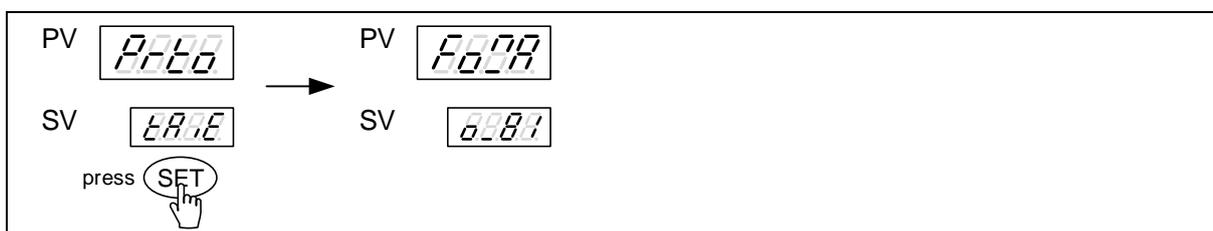
8. Press SHIFT key then lower display will start flash, press UP key or DOWN key to select DATA format then pressing SET key to save the current setting.
