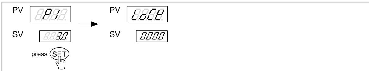
4. Set LOCK to 1000, press SET key + SHIFT key for 3 seconds to enter Level 5
