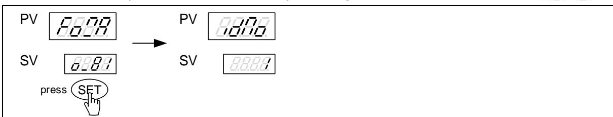
10. Press SHIFT key then lower display will start flash, press UP key or DOWN key to select slave address then pressing SET key to save the current setting.
