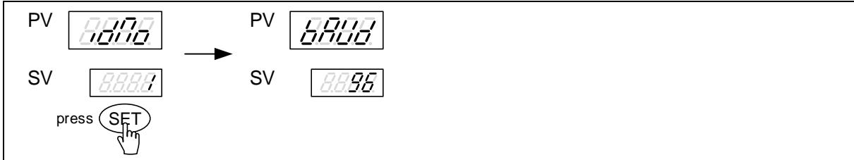
12. Press SHIFT key then lower display will start flash, press UP key or DOWN key to select baud rate then pressing SET key to save the current setting.
