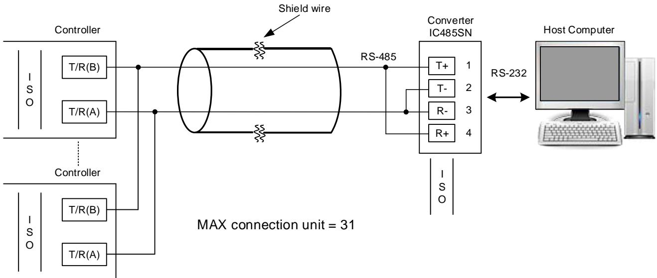
※ The spanning distance for controller connection PC Cable should not be more than 1200 meters.
