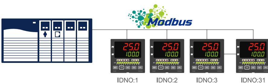
Compatible with Modbus RTU communication protocol to quickly establish links with HMI, PLC or SCADA software.
