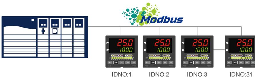
Compatible with Modbus RTU communication protocol to quickly establish links with HMI, PLC or SCADA software.
